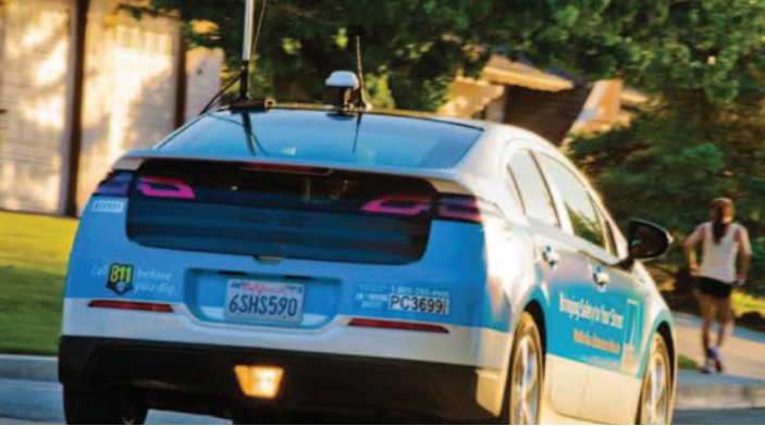
Pacific Gas and Electric Company (PG&E) conducts ongoing gas system leak detection surveys using ultra-sensitive methane detection equipment attached to cars. Photo Credit: PG&E
